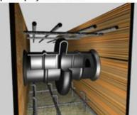
The unique water stop collar acts like an expansion joint, adjusting (up to 1/2" - 12.7mm) to the thickness of the wall. In addition, nailer end caps may be nailed to concrete forms while they also form a smooth beveled finish between wall and formed hole.
