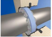
Century-Line® Model CS Sleeves are ideal for poured wall construction. Made of HDPE thermoplastic, they are lightweight and easy to handle. Molded-in waterstop and reinforcing ribs serve to anchor the sleeve in the wall and resist pour forces. Nailer end caps are provided to make placement in forms simple and accurate. Sleeves are available in 16 diameters, up to 25", and any length. In the event of a field change they can be shortened with ordinary hand tools.
